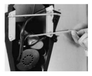
6 As soon as the second pin is removed, be sure to hold onto the gearmotor as it slides forward. Then place the gearmotor aside.
